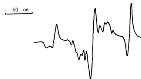
Fig. 1-B. ESR spectrum obtained by \alpha -naphthol photosensitization of methanol (irradiated by <3100 \text{ \AA} at 77^\circ\text{K} ).
